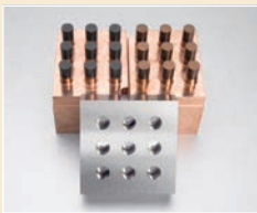
Multi-hole Machining by Intricate Electrode
